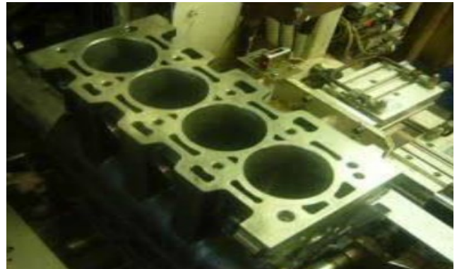
The problem of cylinder block cleanliness was identified as the problem that required rework activities.
