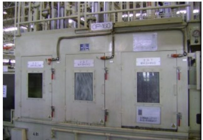
OP#16 machine is for washing process of cylinder block.
