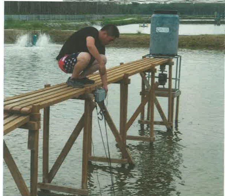
LDMS placed sensors in the ponds to monitor the water quality
